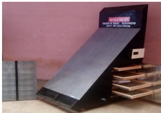
Fig.8 Fully constructed solar tunnel dryer
